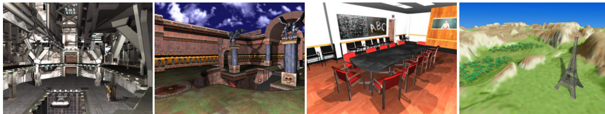
Several example scenes rendered in realtime with 20 to 60 frames per second on the SaarCOR prototype hardware. From left to right: UT2003, Quake3, Conference and Terrain. Adding support for dynamically modifying these scenes actually reduces the hardware requirements.
